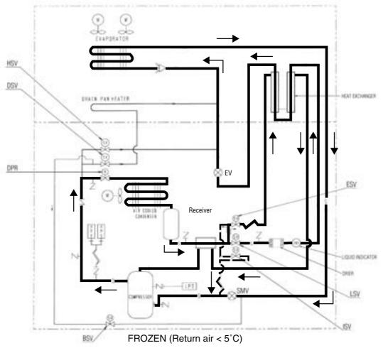
EV :Electronic Expansion Valve LSV :Liquid Solenoid Valve DSV :Defrost Solenoid Valve ESV :Economizer Solenoid Valve DPR :Discharge pressure regulator SMV:Suction Modulation Valve
