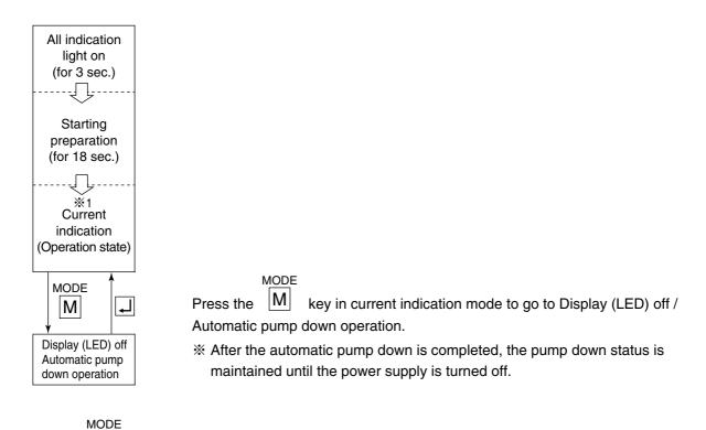
Pressing the M key changes the mode between Display (LED) off and automatic pump down. The set point can be set by using  $\bigtriangleup$  key or  $\bigtriangledown$  key.
