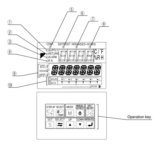
① SUPPLY LED (Lights when "supply air temperature" is indicated.)
