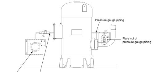
Low pressure gauge Pressure gauge piping
