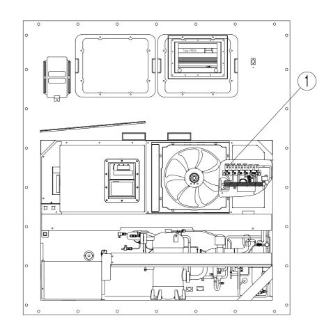
① Reheat coil solenoid valve (RSV)
