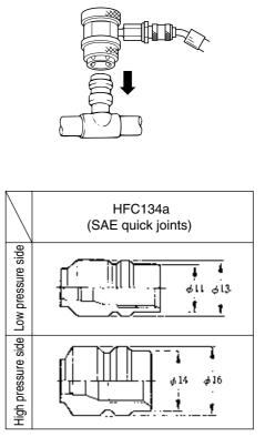
Be sure to use the gauge manifold with the quick joints shown above.
