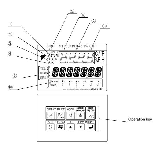
① SUPPLY LED (Lights when "supply air temperature" is indicated.) ② RETURN LED (Lights when "return air temperature" is indicated.)
