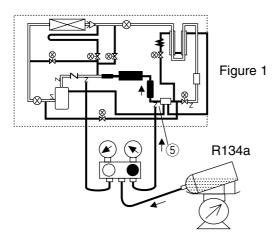
2.Replace the manifold gauge hose to port ③ and add the liquid refrigerant. Then if it reached to the specified amount close the cock of the refrigerent cylinder.
