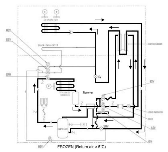
EV:Elec.Exp.Valve LSV:Liquid Solenoid Valve DSV:Defrost Solenoid Valve ESV:Economizer Solenoid Valve DPR:Discharge pressure regulator SMV:Suction Modulation Valve HSV:Hot Gas Solenoid Valve ISV:Injection Solenoid Valve BSV:Discharge gas Bypass Solenoid Valve LPT:Low Pressure Transducer HPT:High Pressure Transducer HPS:High Pressure Switch
