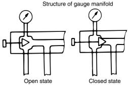
Open and closed states of gauge manifold
