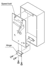
④Replace the temperature recorder board.⑤After replacement, be sure to check the wiring and operation.
