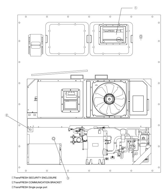
•An example of installation of CA devices, inside
