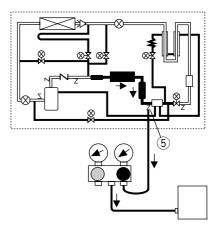
③Recover completely refrigerant left in the unit from ports ④ & ⑤.
