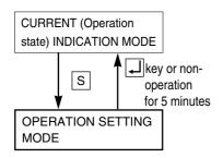
To change to the OPERATION SETTING MODE, press the S key while the unit is in the CURRENT INDICATION MODE.
