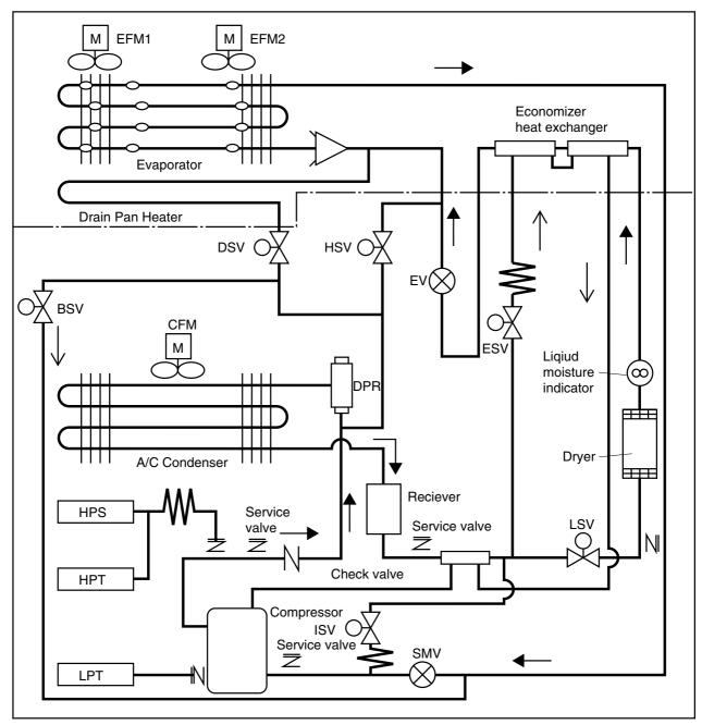
EV :Electronic Expansion Valve LSV:Liquid Solenoid Valve DSV:Defrost Solenoid Valve ESV:Economizer Solenoid Valve SMV:Suction Modulation Valve
