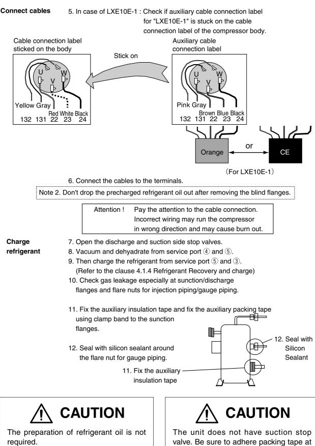
The compressor has been charge with the oil.
