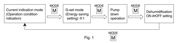
%1: When the dehumidification ON-A · OFF is set to ON, G-Set operating mode will be skipped.
