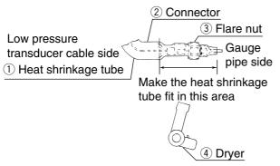
⑦ Apply sealer between the heat shrinkage tube and the flare nut. (Sealer :KE4898)
