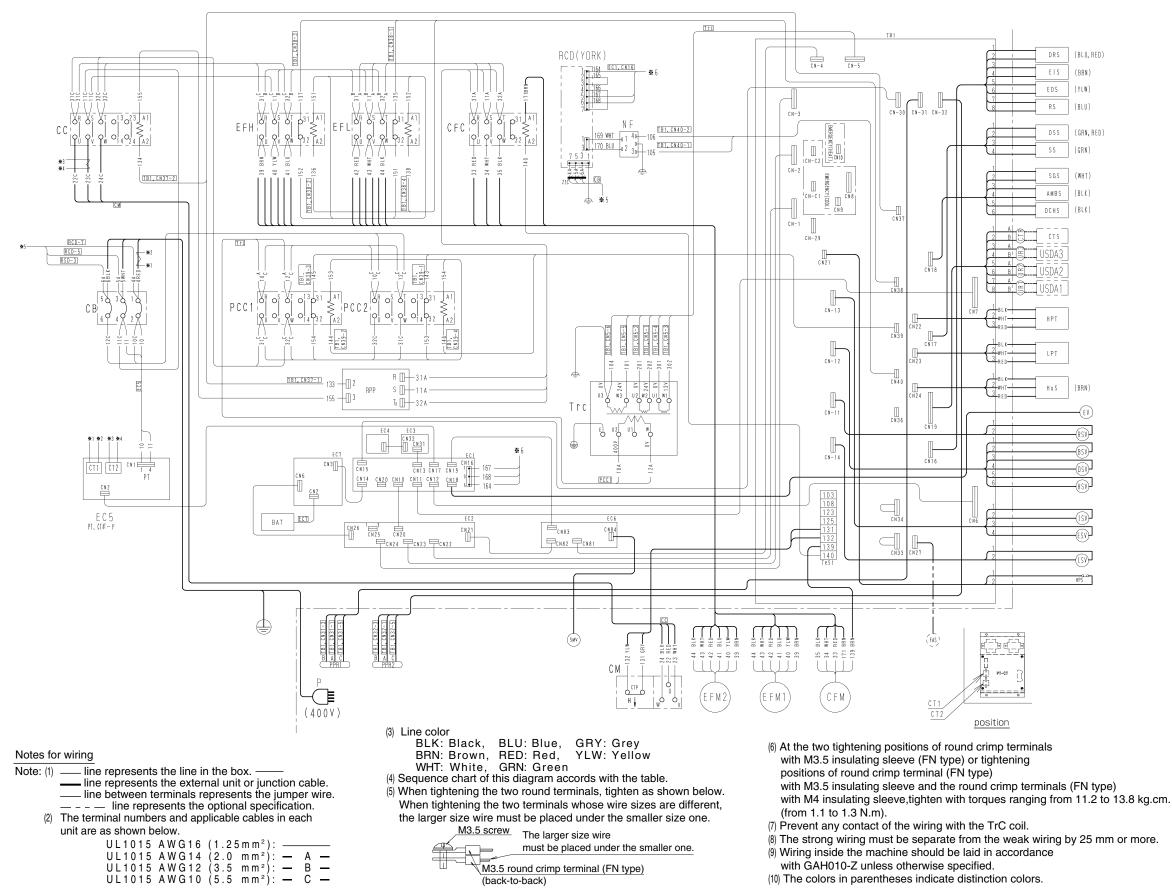
7.15 Schematic wiring diagram (Connector type terminal board, temperature recorder and dry battery)
