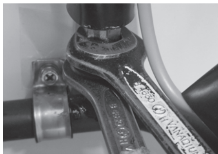
Fig. 1 Use two wrenches when removing and installing.
