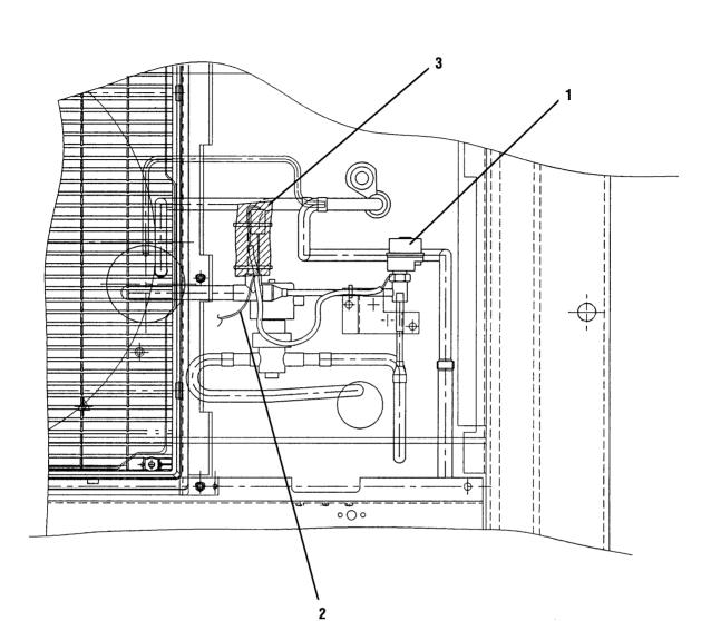
Parts related with the option 1-Moter operated valve coil with junction connector オプション関連部品 1 一震動会コイル(中継コネクタ付)
